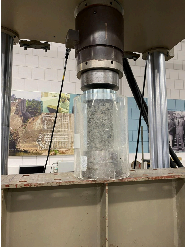
Figure 5. Image of the MTS 810. This image depicts the MTS 810 load frame which was used to test the samples. Also pictured is one concrete sample before any force was applied. Each sample was tested using the MTS and data was collected each second measuring force applied and displacement. Image by author.
